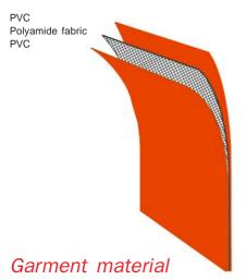
Strong and flexible polyamide fabric coated on each side with PVC.
