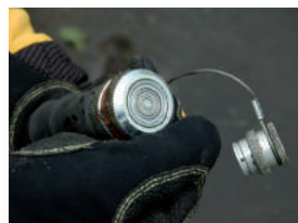
- no dirt inside couplers
