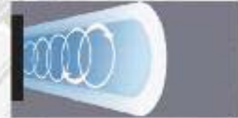
Standard Shroud Airflow is more diffused
