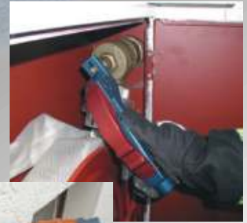
Wrench with key width 7+8+11 mm e.g. usage on wall hydrant or gas tap etc. if the hand wheel is missing
