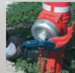
Opening / closing of hydrant closure covers (cover capsule) by DIN 3223
