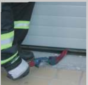
Lever tip, breaker tool, elongated by UNI-combined grip - up to 500 Nm - support points for controlled force transmission - easy entering and widening of gabs, to lift or break open Example: Opening of doors / Opening of gates
