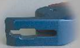
Wrench with key width 7+8+11 mm e.g. usage on wall hydrant or gas tap etc. if the hand wheel is missing
