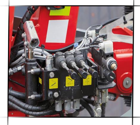
The unit is controlled by a lever and switches located on its main body, accessible from ground level.
